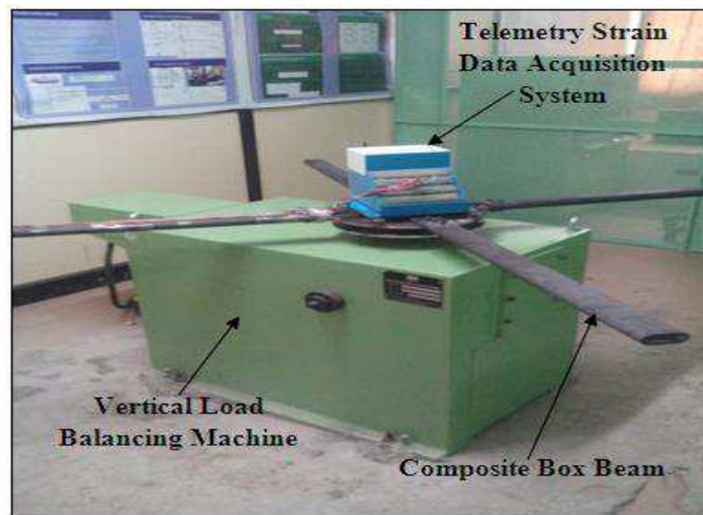
Figure 5.1 Experimental setup for Rotating Analysis of Composite Blade
