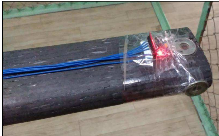
Figure 5.4 Accelerometer GY-521 mounting on free end of composite blade
