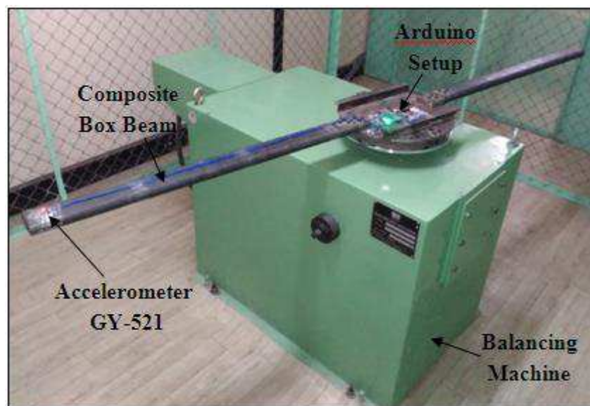
Figure 5.3 Experimental setup for acceleration in rotating composite blade using GY-521 Accelerometer
