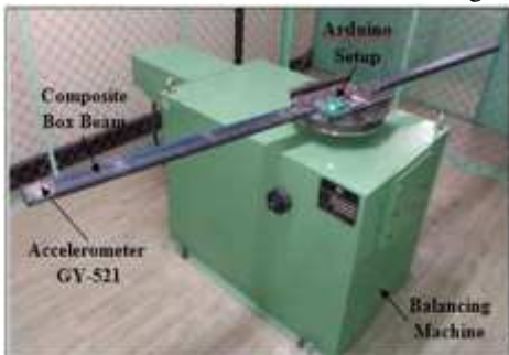
Figure 8 Experimental setup using GY-521 Accelerometer
